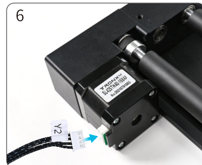
Plug the other end of the motor cable into the Y-axis device motor
