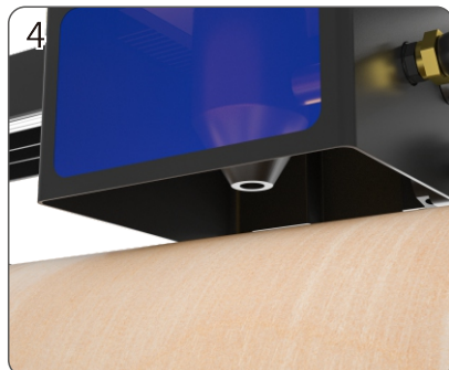
Move the laser forward so that the laser outlet is on the highest surface of the carved object
